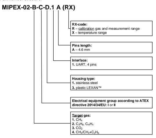
Term **target gas** refers to LED and photodiode spectral range, which is adjusted for best detection of a certain gas, while term **calibration gas** refers to gas mixture used for sensor calibration.
